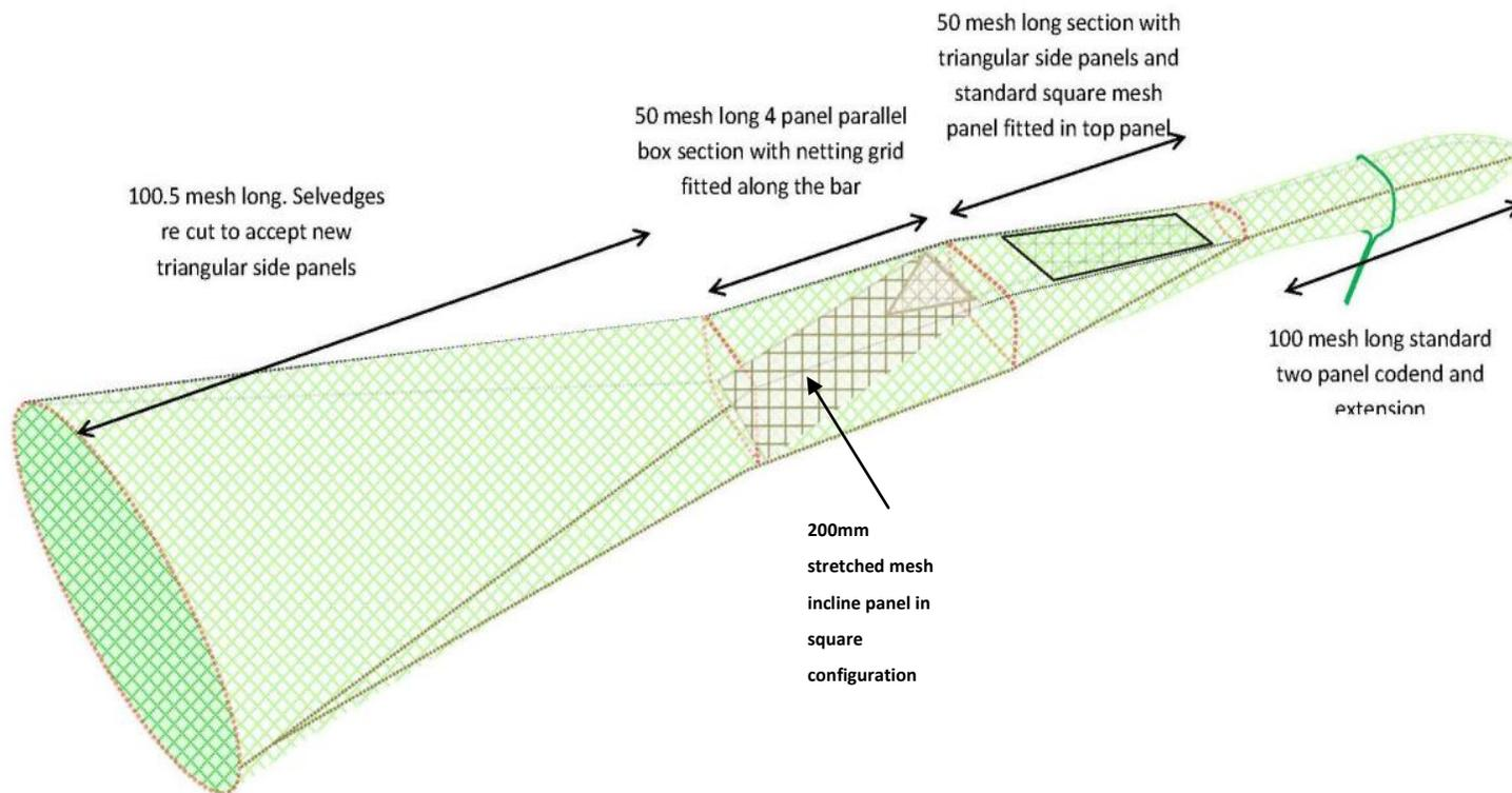
Figure 3 Net Grid modified design 2 short version (illustration by Mike Montgomerie, Seafish).
