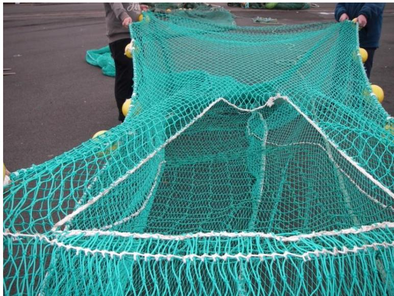
Figure 6 Escape hole and incline panel.
