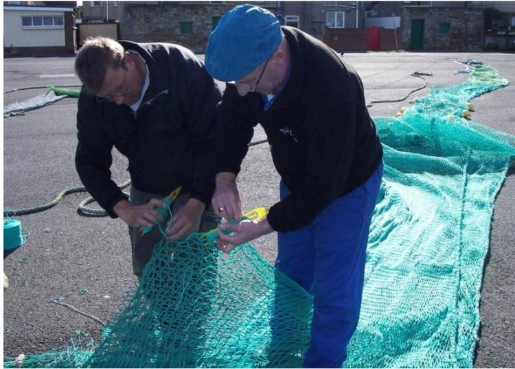
Figure 5 Skipper and Cefas SIC inserting Net Grid.
