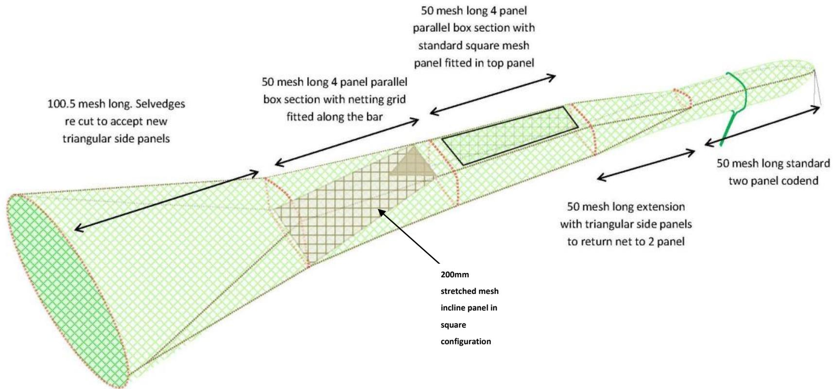
Figure 2 Net Grid modified design 1 long version (illustration by Mike Montgomerie, Seafish).
