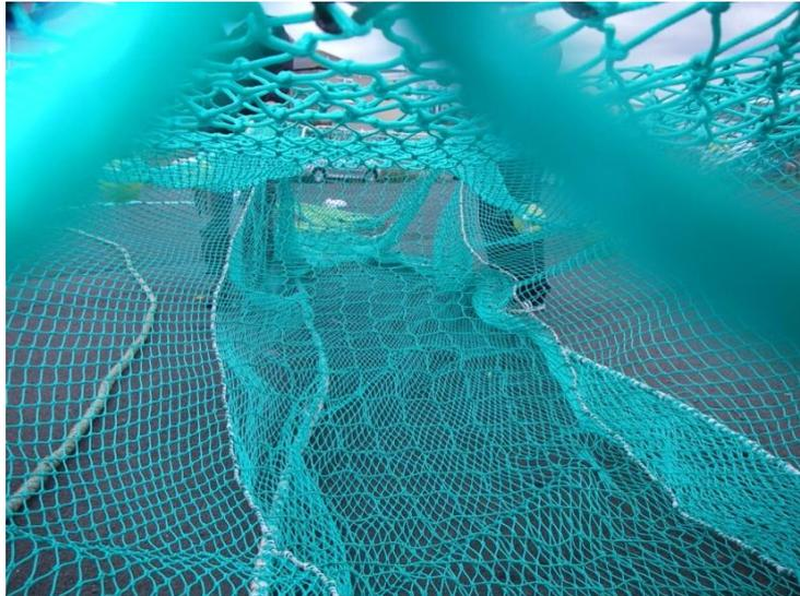
Figure 7 Escape hole and incline panel interior of net view.
