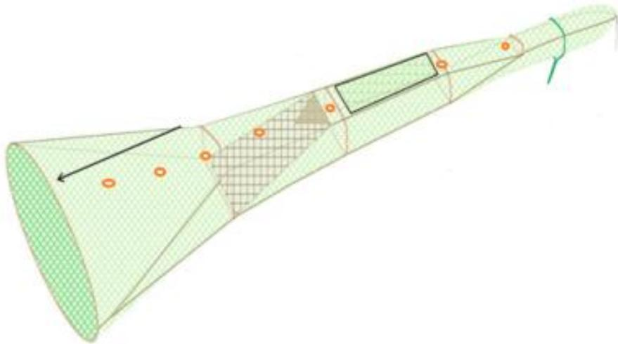
Figure 22 Positions of Scanmar® pitch and tilt sensor placement (orange circle)
