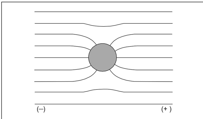
FIGURE 6 Distorted electric field around a spherical particle
