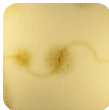
Appearance of the patch with defect visible as a snowflake pattern
