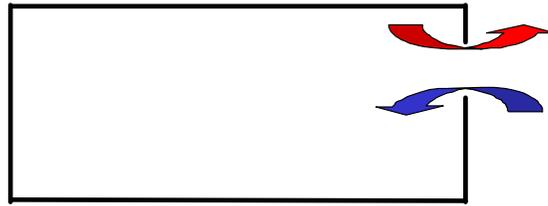
**Figure 1(a) Single sided ventilation: a single openable window or vent**
