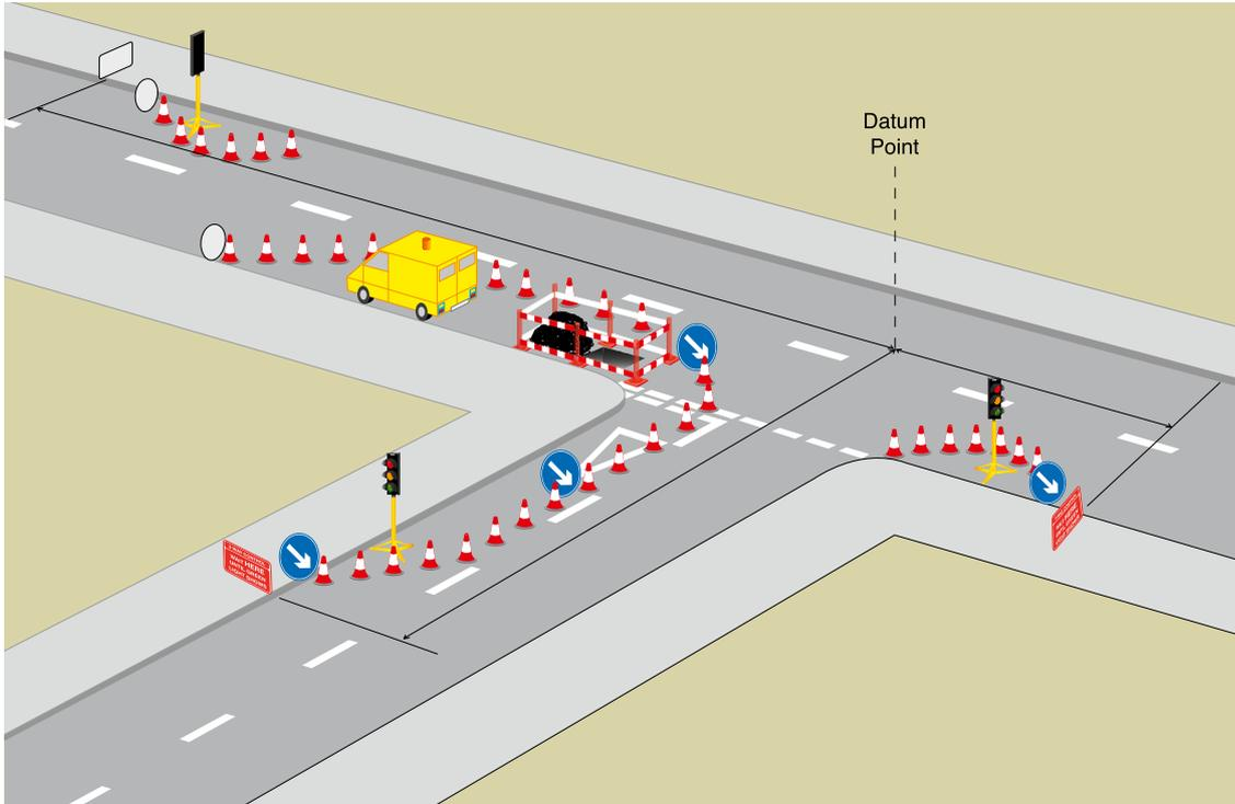
**Datum point** (Note: The Chapter 8 triangular warning signs, guarding on the footway and possible secondary signals have been omitted for clarity.)
