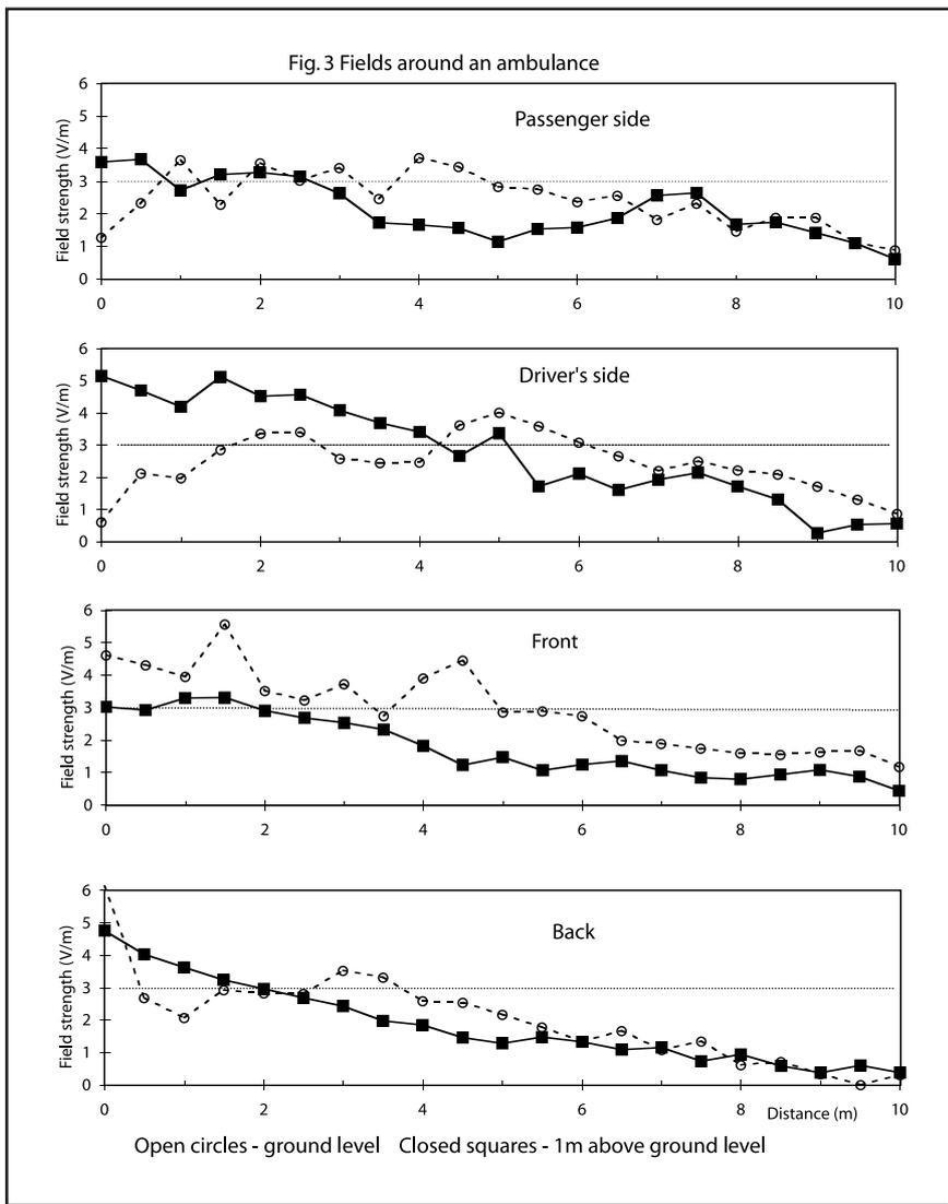
to the ambulance the field distribution near the ground is dominated by the screening effects of the metal in the vehicle body.
