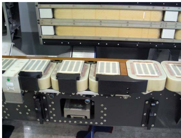
Figure 3: Lift magnets and lateral location system
