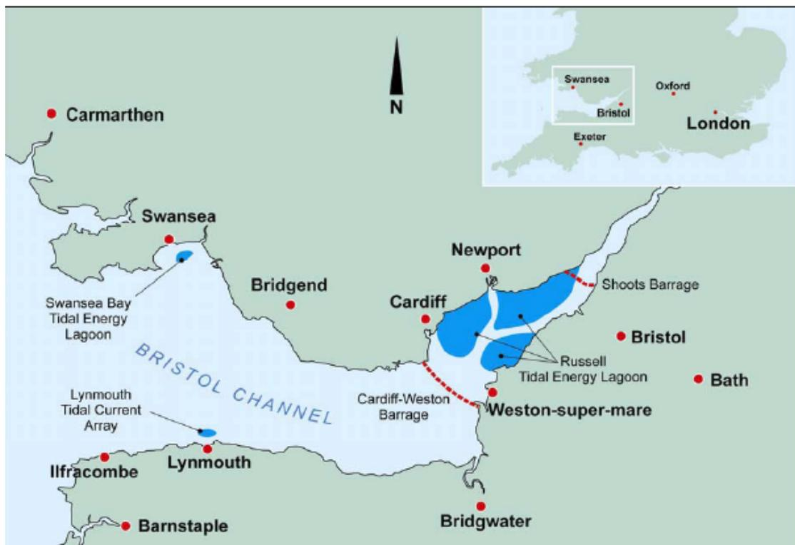
**Figure 1.1** Location of the Russell Tidal Energy Lagoons, the Swansea Bay Lagoon and the Lynmouth Tidal Current Array. The position of the Cardiff-Weston and Shoots tidal energy barrages are shown for comparison.
