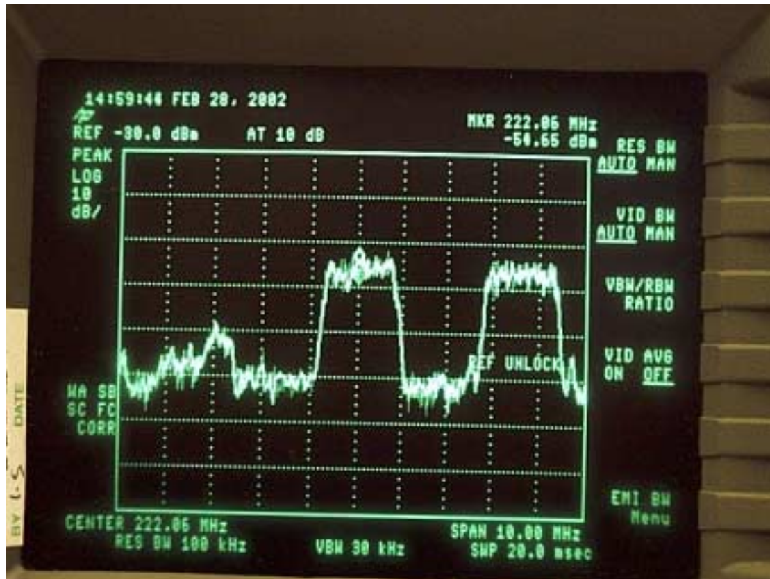
Figure 4.16: The DAB multiplex with no interference signal
