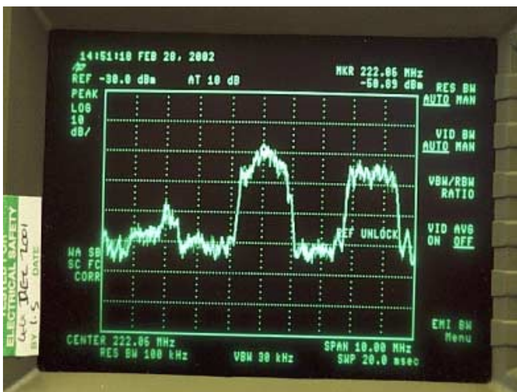
Figure 4.18: DAB multiplex with the Lexmark interfering signal sufficient to cause the DAB receiver to mute its audio output
