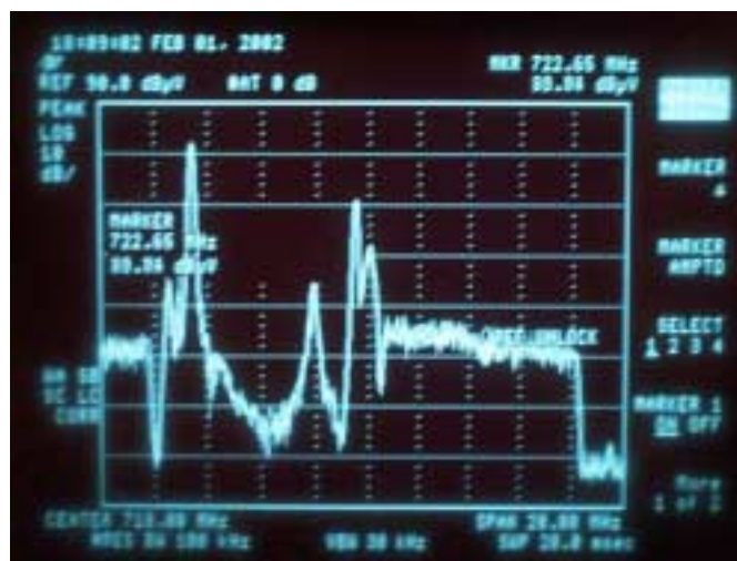
Figure 4.2: Off-air signal (measured at RF feed from mast-head amplifier – reduced by 11.8 dB for spectrum at STB)
