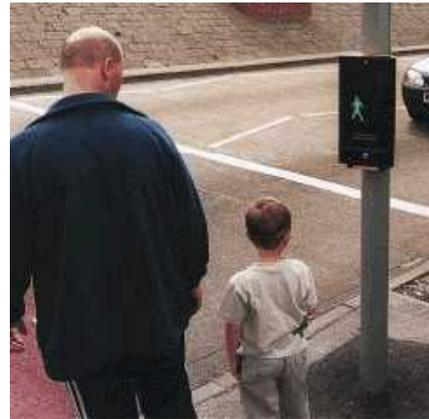
At some sites a single straight crossing with a central island may be feasible. Additional pedestrian on-crossing detectors may be required at some sites to ensure that pedestrians continue to be detected over the whole crossing area. The pedestrian demand unit should be installed on both sides of any central refuge island, to enable pedestrians waiting in this area to register a demand. The use of one or more kerbside detectors within this area is also recommended.
