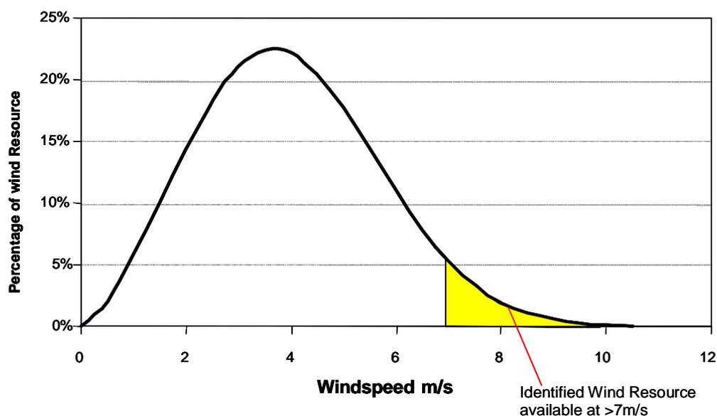
By converting this into a cumulative probability distribution, we are then able to determine the share of the total wind resource that occurs between different wind speeds. This wind resource is then divided between large and small wind farms, 80MW and 30MW respectively. If there is insufficient wind resource for an 80MW wind farm at a given wind speed then a 30MW wind farm is selected. These sizes
