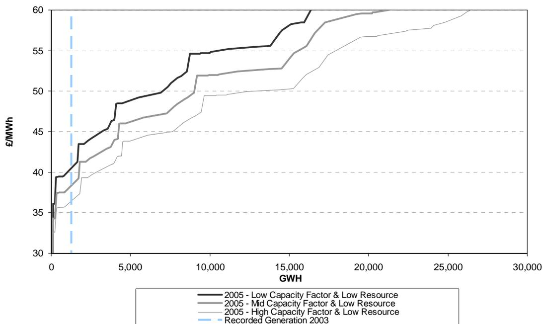
Figure 3.9 Wind supply curve capacity factor sensitivity (high resource scenario)
