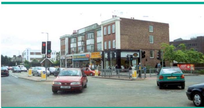
If the number of right-turners exceeds the number that can clear the junction in gaps, or during the intergreen, special provision will probably be required. Note that if right-turners are left in front of the stop line after a change to another stage, not only will the driver feel in a vulnerable position but the presence of the vehicle may obstruct pedestrians wishing to cross.
