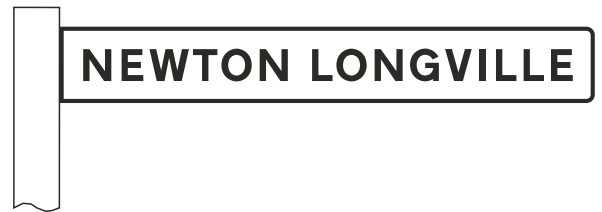
Fingerpost signs: design prescribed in Traffic Signs Regulations 2002 (Diagram 2141)
