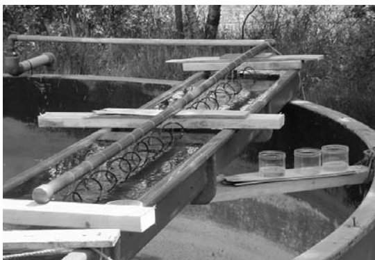
Temporary raceway set up at hatchery for maintenance of sediment pots.
