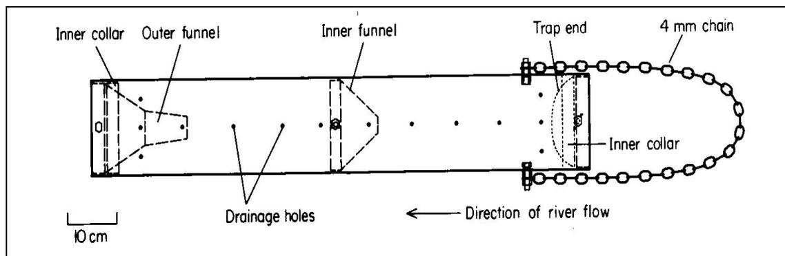
**Figure 4. Trap design developed by Morris and Maitland (1987).** This particular model has both an outer and an inner funnel. The sampling tubes were made of UPVC domestic waste discharge pipe (approximately 15 cm in diameter).
