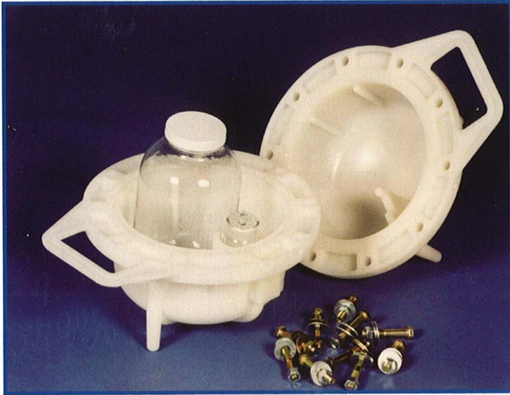
Figure 7 - Single CAIS Assess and Neutralization System
