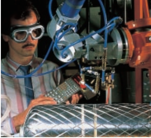
A technician operates a robotically mounted laser which is being used to weld glass fibre and plastic onto a composite material.
