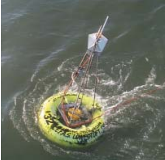
Smart buoy – providing real-time monitoring of the marine environment © Crown copyright, reproduced by permission of CEFAS, Lowestoft
