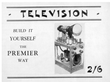
Fig. 5.27 Post-war television receiver kit based on ex-government components
