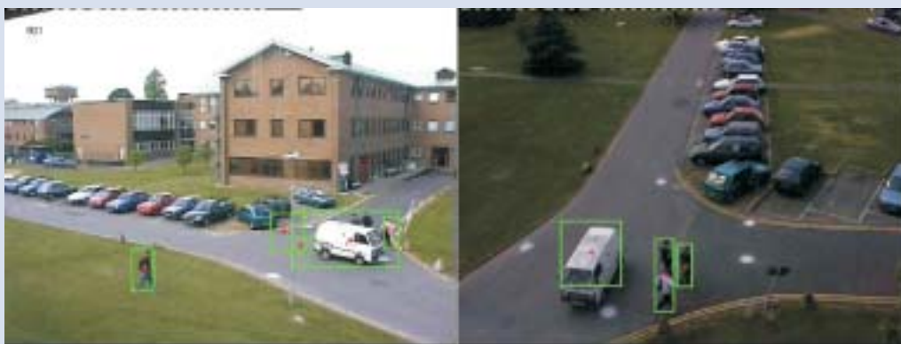
Two camera views, taken from the PETS2001 video sequence. The green bounding boxes locate objects detected in each view. The red dots correspond objects seen in each view using the homography. Image quality and resolution is limited by the JPEG encoding of the image frames.
