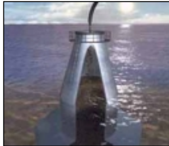
Gravity base foundation picture: Corus
