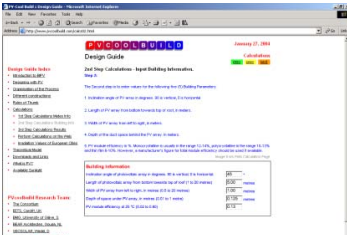
Figure 7: The Second step is to enter values for the following five Building Parameters
