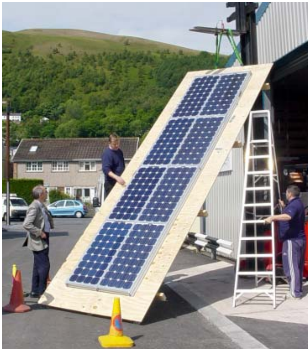
Figure 3: EETS variable angle outdoor test facility.
