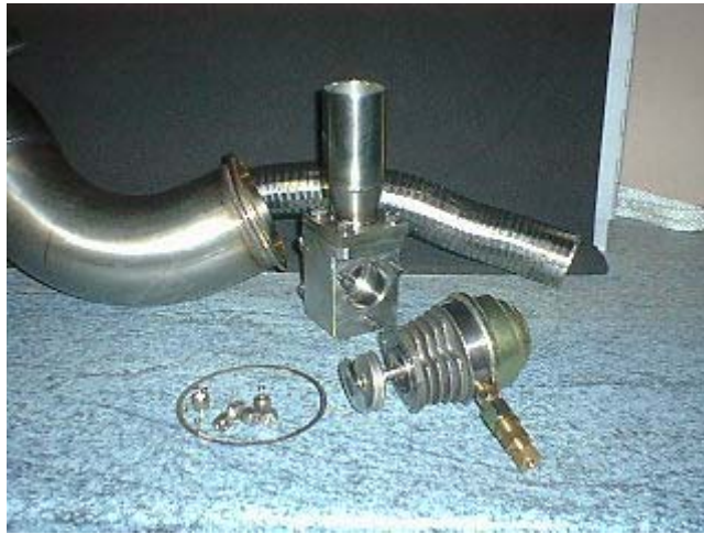
Photo 3.2.3: Turbine Pressure Relief Valve
