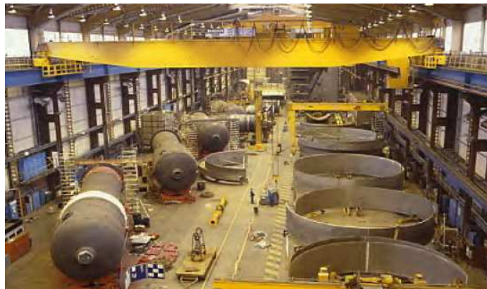
Figure 13 – Steam Generator fabrication at Mitsui (now Doosan) Babcock, Renfrew, for Sizewell B. (Courtesy of Doosan Babcock Energy Ltd.).
