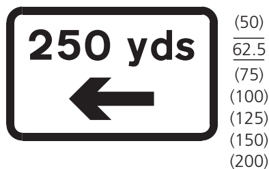
573 Distance and direction to hazard
