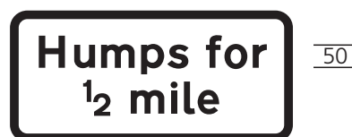
557.2 Road humps for the distance indicated
