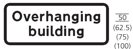
530.1 Building overhanging part of carriageway
