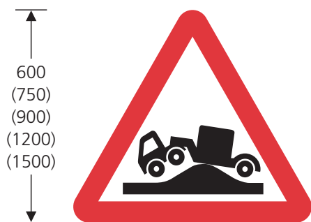
782 Risk of grounding
