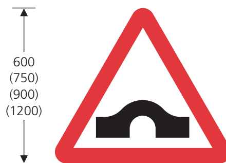
528 Hump bridge ahead
