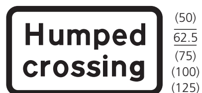
547.8 Zebra crossing or signal-controlled crossing on road hump ahead
