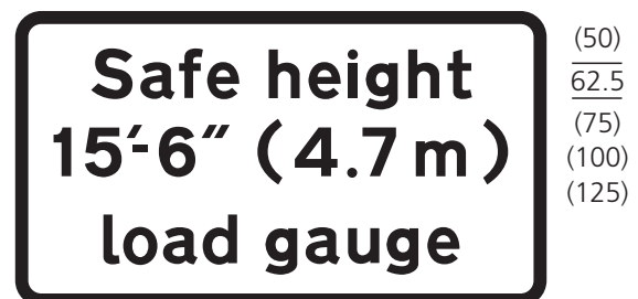
780.2A Load gauge and safe height beneath cable
