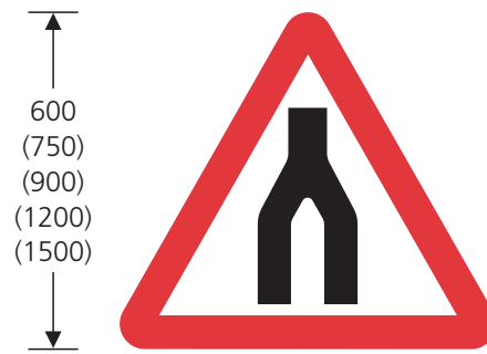
520 Dual carriageway ends ahead
