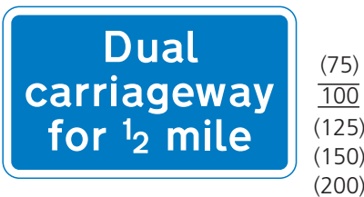
818.1A Short length of dual carriageway beginning directly ahead
