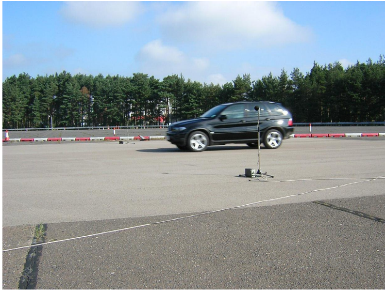
Figure 4.4: A tyre noise test on the ISO surface
