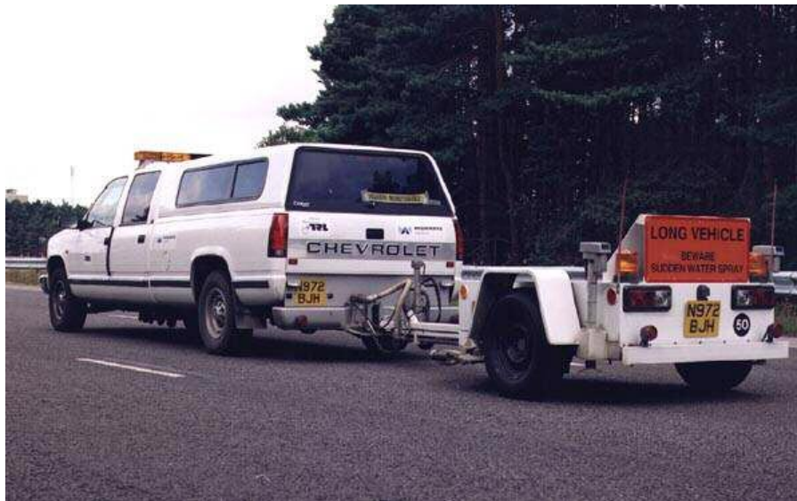
Figure 4.3: The TRL pavement friction tester
