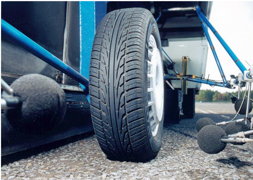
Figure 7.3: Test tyre and microphone set-up in TRITON’s enclosure
