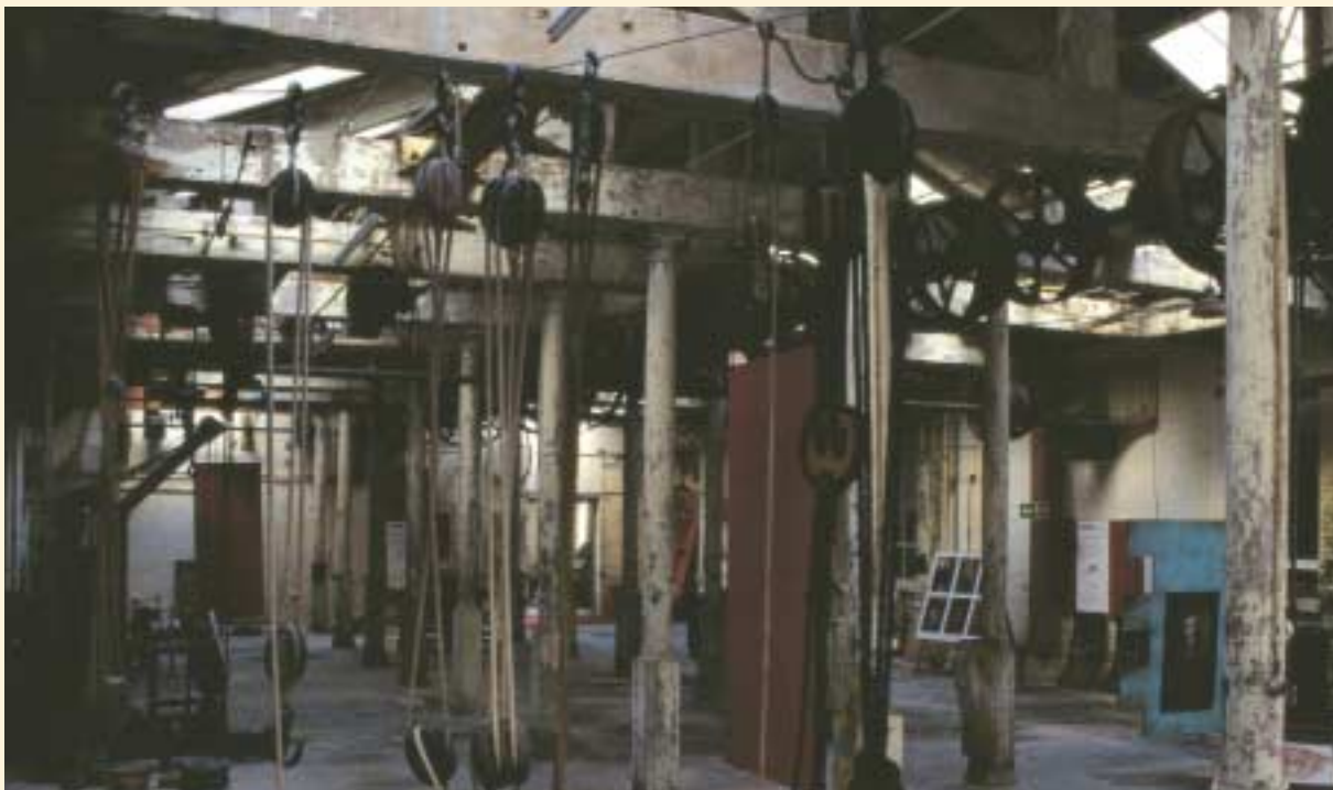
Ground floor of the Block Mills, showing some of the surviving block-making machinery
