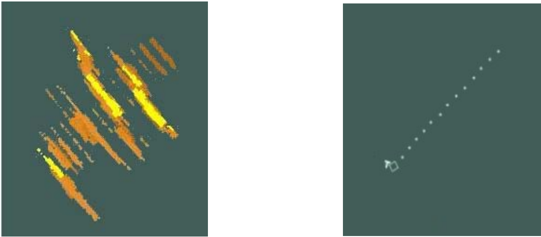
Figure 2. A Processed Video output is shown on the left and a plot extracted output is shown on the right. The target is moving from top right to bottom left in both pictures.
