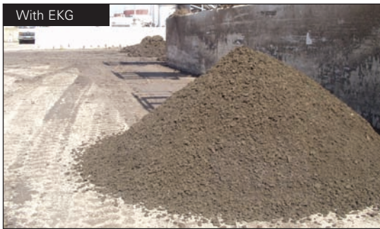
Application of EKG technology to a standard belt filter press raised the solids content of dewatered sludge from 20% to 33% resulting in major reductions in volume and improvement in strength
