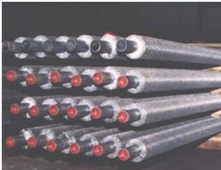
Figure 5: Finned tube bundle (Courtesy of Mitsui Babcock Energy Ltd).
