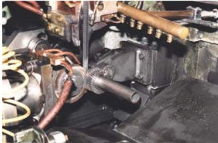
Figure 4: Finned tube manufacture (Courtesy of Mitsui Babcock Energy Ltd).
